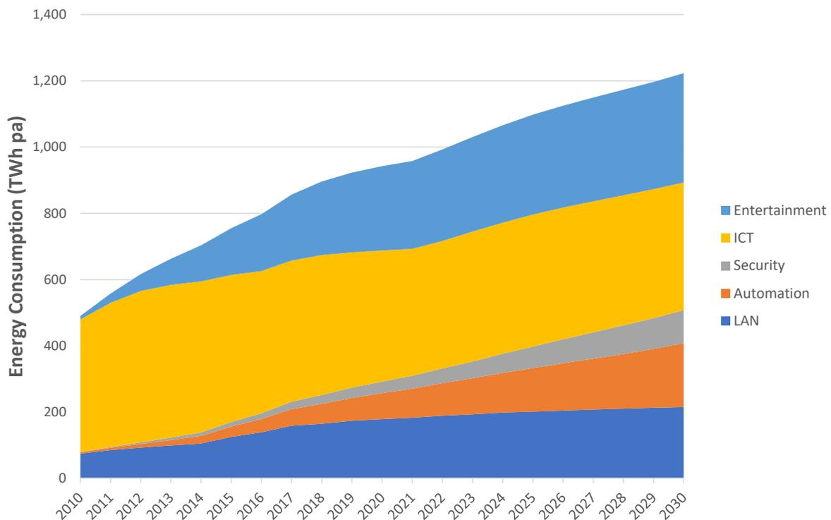
The total energy consumption shown in Figure 12 is higher than in TEM1.0, as it now includes the energy consumption of displays when edge devices receiving video streaming services. This difference can be clearly observed by the increase in energy consumption of the entertainment category of devices compared to the estimates in the TEM1.0 for the same category.
