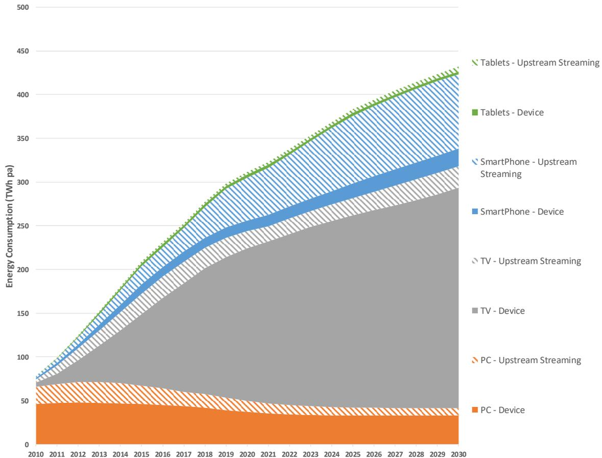
Figure 6 highlights the relative portions of the streaming media traffic and non-streaming upstream traffic energy use. The downward trend, starting in 2014, in streaming media and non-streaming traffic energy use reflects the improvement in the efficiency of DC and WAN equipment (i.e., servers, routers, switches, etc.).
