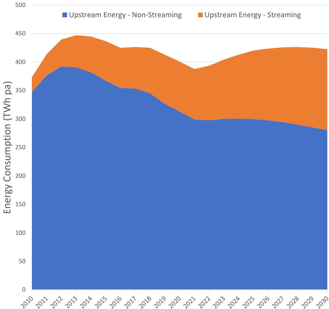
Figure 7 shows the energy consumption of the principal components associated with streaming media traffic and non-streaming traffic and connected devices. It reveals that the upstream streaming traffic component is the smallest.
